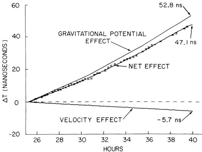
Fig. 47. Growth of the proper time integral during flight.
