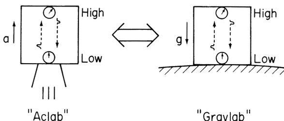
Fig. 14. Implication of the Principle of Equivalence for the behavior of clocks in a gravitational field.
