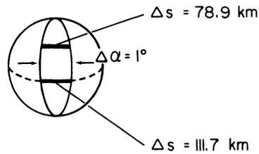
Fig. 19. Different proper distances on the sphere.
