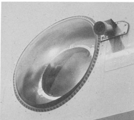
Fig. 41. Optical corner reflector next to a forward observing window.
