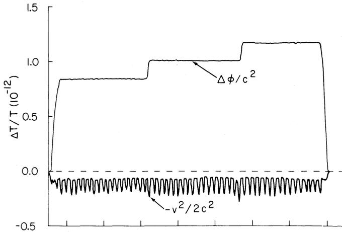
Fig. 46. Radar tracking data converted to  $\Delta\phi/c^2$  and  $-v^2/2c^2$ .
