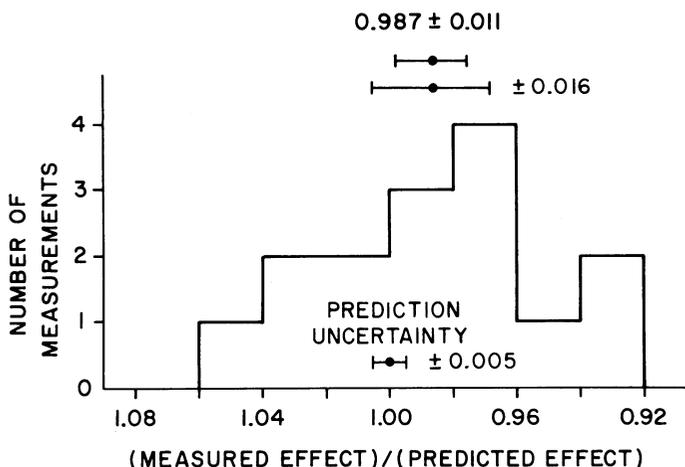
Fig. 50. Histogram of 15 measurements: three cesium beam clocks on each of five flights.
