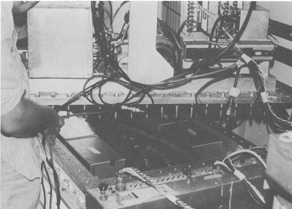
Fig. 37. A "clock box" used to shield the clocks from environmental changes.
