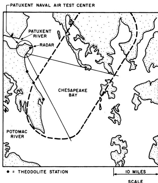
Fig. 24. Approximate path of the aircraft over the Chesapeake Bay.
