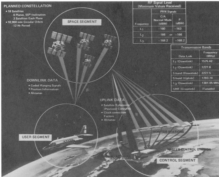
Fig. 61. How the Global Positioning System works.
