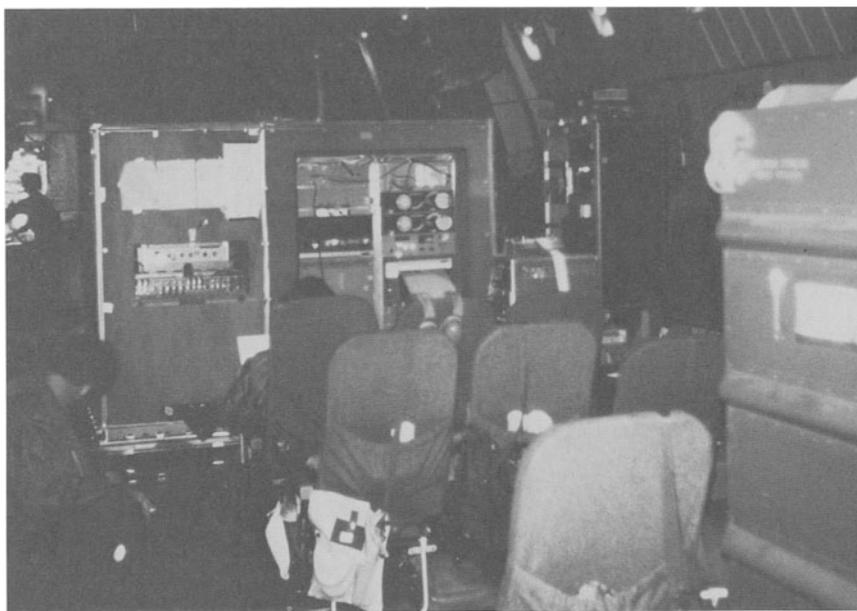
Fig. 56. Installed clock assembly during a flight. The seats are for the travelling "clock-watchers."
