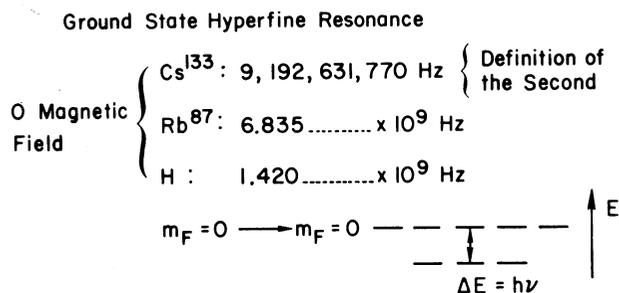
Fig. 28. Frequencies used in modern atomic clocks.
