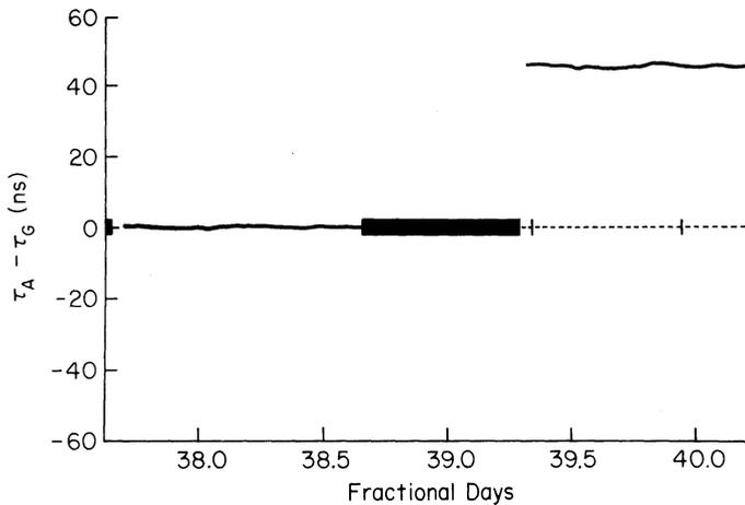
Fig. 49. Comparison of Flying Clock #3 to the average of ground clocks shows relativistic time difference after flight.
