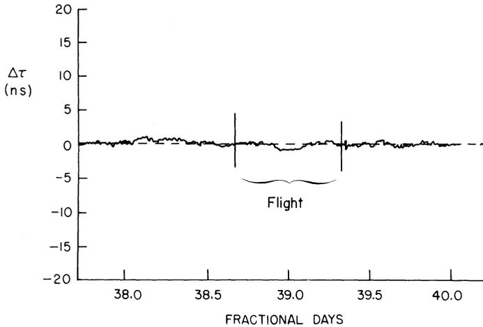
Fig. 48. Comparison of Flying Clock #3 to the average of all flying clocks shows no discernable effect of flight.
