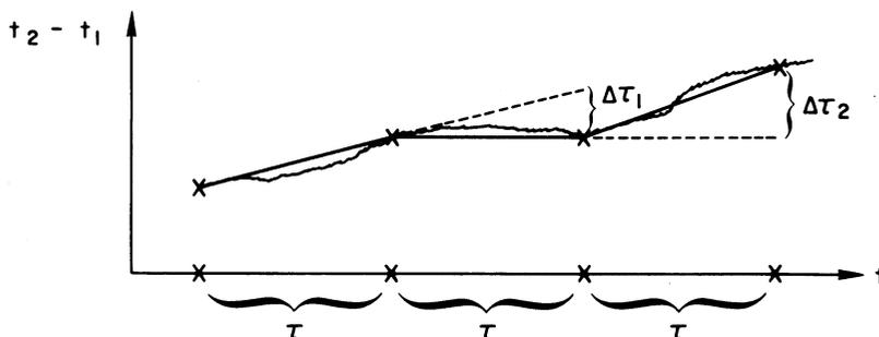
Fig. 33. Illustrating the definition of the Allan variance  $(\Delta\tau)_{\text{rms}}/\tau \equiv \sigma(2;\tau)$  used to describe the behavior of two atomic clocks.
