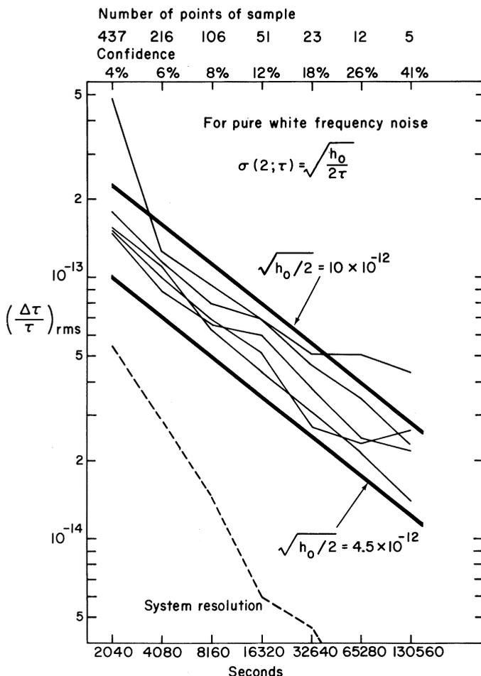
Fig. 35. Measured fractional stability of the cesium beam clocks used in the experiment.
