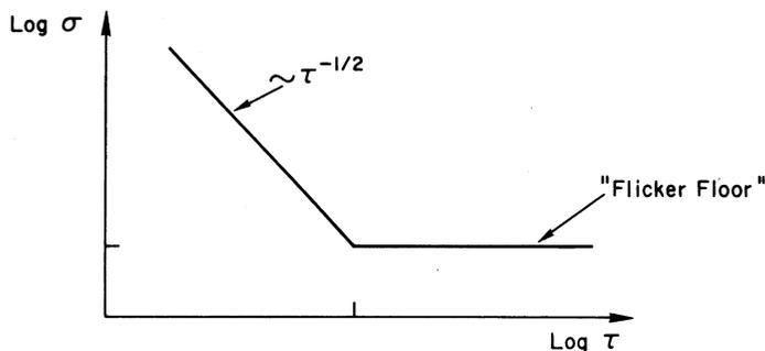
Fig. 34. Illustrating the occurrence of a lower bound to the fractional stability of clocks.
