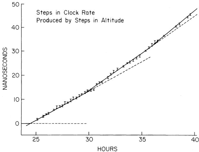
Fig. 45. The atomic clock as an altimeter.
