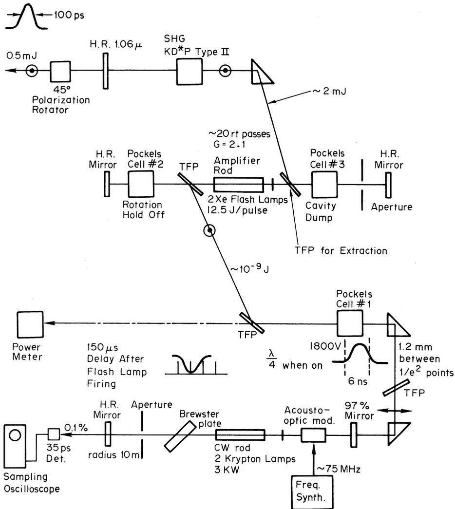
Fig. 27. Diagram of the neodymium YAG laser with mode-locking, multi-pass amplification, and frequency doubling.
