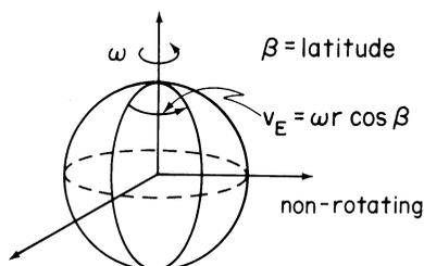
Fig. 26. Inertial system centered on earth used for evaluating the proper time interval.
