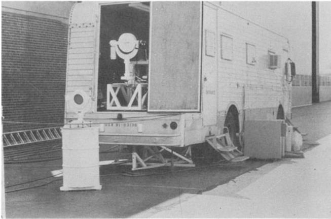
Fig. 40. Laser beam directing optics and bus containing laser, receiving telescope and photodetector.
