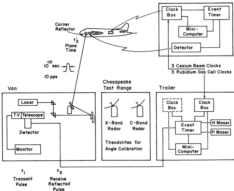
Fig. 22. Schematic diagram of the local flights with laser pulse time comparisons.
